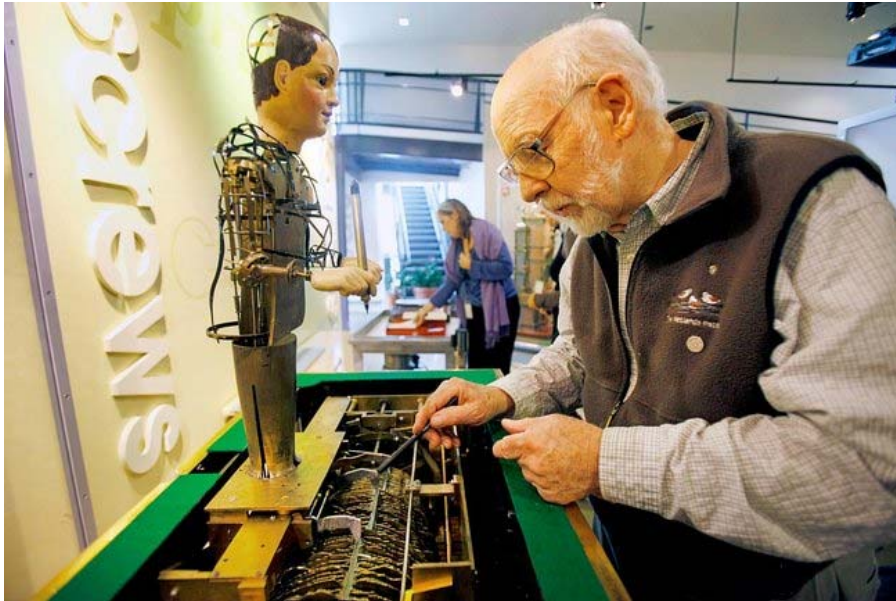
INTRICATE Charles F. Penniman oversees the movement of the automaton's many cams, which function as its read-only memory.
